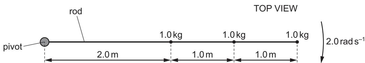
The rod rotates in a horizontal plane about a pivot at a constant angular velocity of  $2.0 \text{ rad s}^{-1}$ .
