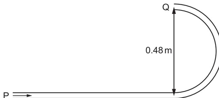
A particle is projected along the tube from the lower end P with a speed of  $4.0 \text{ m s}^{-1}$  so that it just reaches the upper end Q.
