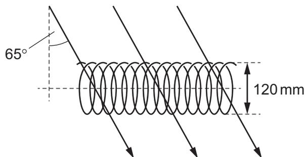
The coil has 240 turns and a diameter of 120 mm.
