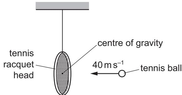
A tennis ball is fired at the centre of gravity of the racquet head at a speed of  $40 \text{ m s}^{-1}$ . The ball bounces from the racquet head in the opposite direction at a speed of  $30 \text{ m s}^{-1}$ .
